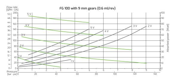
Note: Characteristics with water at 20 °C (68 F) and without relief valve. Fluids different from water must be validated by the Customer. Temperature requirements different from ambient temperature must be mentioned on the order.
