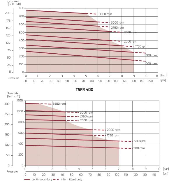
Note: Hydraulic performances measured with 20 °C (68 F) water and without bypass. Curves are averages. For applications involving other fluids, high temperatures, unusual processing conditions or speed higher than 2500 rpm consult the factory or an authorized Fluid-o-Tech distributor.
